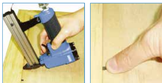
Two ways to fix V nail.
